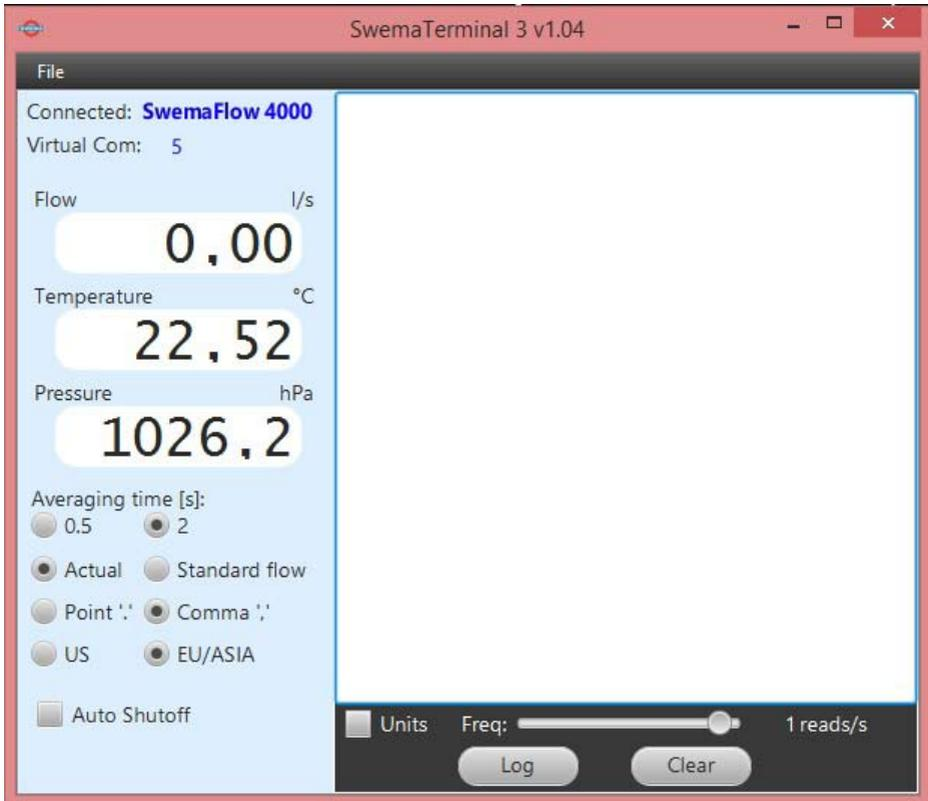
With SwemaTerminal 3 it's possible to change settings, print stored measurements, update firmware, print calibration protocol, do on-line logging and store the logged data on your PC. Information of what kind of instrument and at which COM-port it's connected can be found on the top left side.
