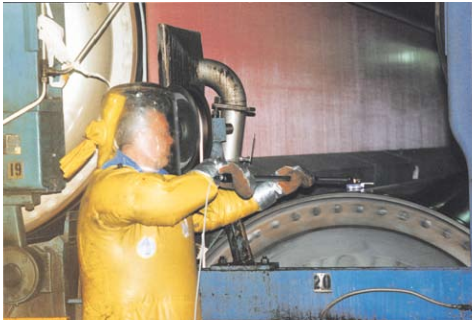
SWT 315, measuring surface temperature of a drying cylinder. A 10m extension cable connects to a Swema 3000 or SwemaTemp 20.
