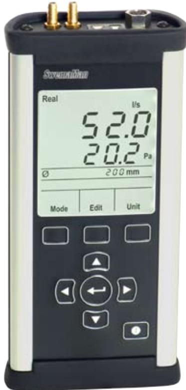
**WARNING! Before start measuring please read chapter "6. Settings (Set)". At delivery k2-factor and automatic density compensating for atmospheric pressure and temperature is turned on.**
