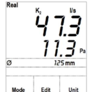
Air flow measuring mode with set diameter.
