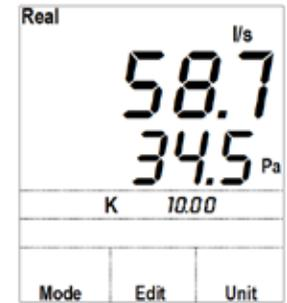
The k-factor SwemaMan 8 is set to measure with is displayed direct under measured pressure.
